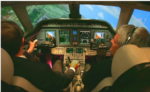
Inside the cockpit of the Citation Sovereign FAA-approved Level D full-flight, full-motion simulator at FlightSafety's Cessna Center in Wichita, Kansas.
